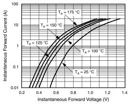
Figure 3. Typical Instantaneous Forward Characteristics
