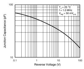
Figure 5. Typical Junction Capacitance
