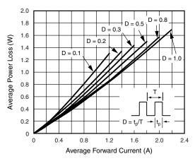
Figure 2. Forward Power Loss Characteristics
