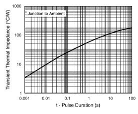
Figure 6. Typical Transient Thermal Impedance
