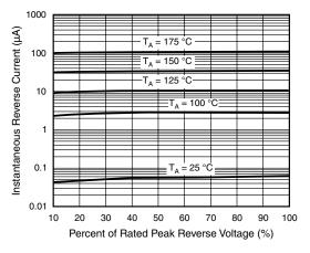
Figure 4. Typical Reverse Characteristics
