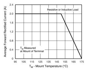
Figure 1. Maximum Forward Current Derating Curve
